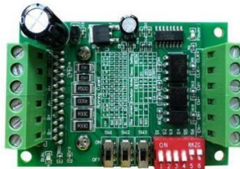
Figure 2 : TB6560 stepper motor driver board
