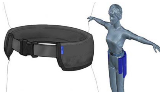
Figure 1. Wearable hip-airbag device protecting patients from being injured due to them falling from having fragile bone structure.
